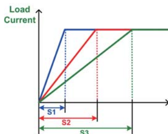
Three different load waveforms of Soft Start Time
